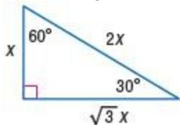
The length of the side opposite the  $60^\circ$  is  $\sqrt{3}x$  and the length of the adjacent side is  $x$ .
