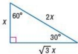
The length of the hypotenuse is  $2x$  and the length of the side adjacent to the  $30^\circ$  angle is  $\sqrt{3}x$ .
