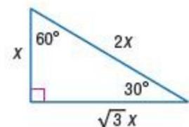
The length of the side opposite the  $60^\circ$  angle is  $\sqrt{3}x$  and the length of the hypotenuse is  $2x$ .
