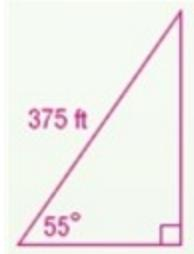
b. Because an acute angle and the length of the hypotenuse are given, you can use the sine function to find the length of the opposite side.
