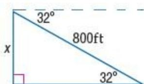
Because an acute angle and the hypotenuse are given, the sine function can be used to find  $x$ .
